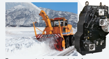
Torque converter type transmission for snow removal vehicles
