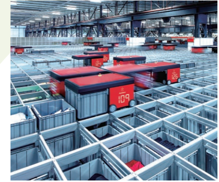
Robot storage systems
