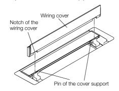
■Opening and closing the wiring cover Hold the outer center of the wiring cover and rotate it while lifting it up. To close, tilt it outward.
