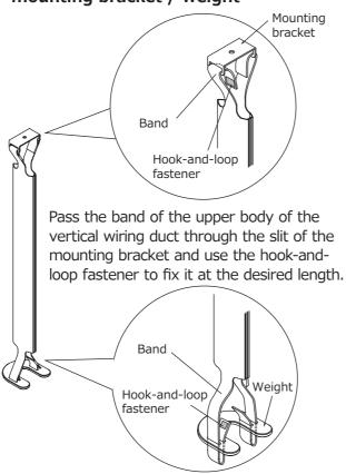
Pass the band of the lower body of the vertical wiring duct through the slit of the weight and use the hook-and-loop fastener to fix it at the desired length.
