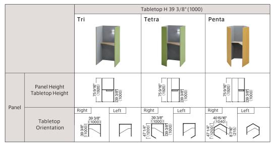
The code for the left type and right type of Tri and Penta is the same. Variation with 75 9/16" (1920) high panels would need lighting on the desk or from the ceiling. We recommend using a non-swivel chair for Tetra and
