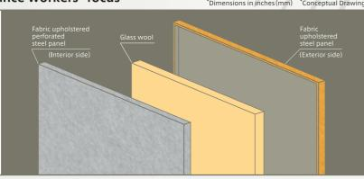
The slim profile panels are only 1 3/16"(30) thick. The core of these panels have glass wool insulation for excellent sound absorption. The clean and straightforward design creates mini-environments for focus throughout the office while also adding aesthetic interest points and color to the workplace.
