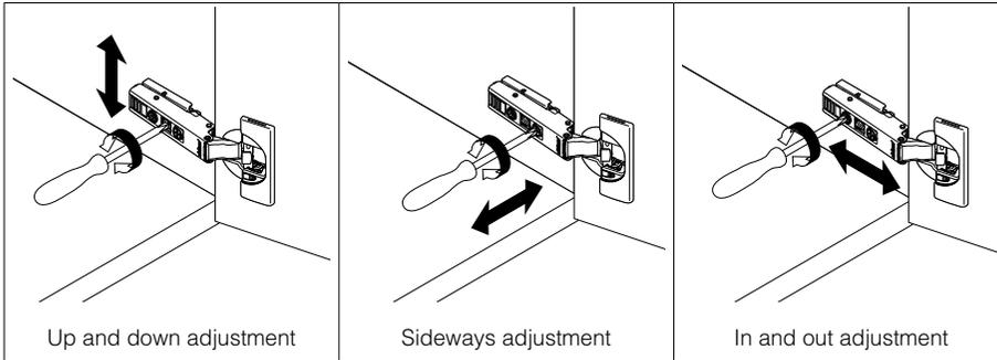
The door hinges can be adjusted in three ways.
