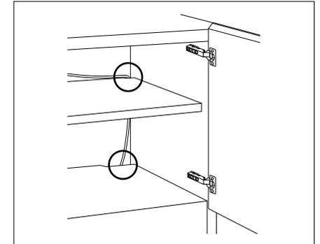
Cable openings are provided at the bottom boards, the shelves, and the dividers for clean cable management.
