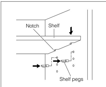
The shelf height can be adjusted on 1 1/4" increments.
