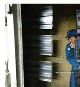
Spraying the agent by hand during the pre-treatment process and confirming its effect
