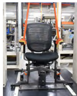
Armrest durability test according to BIFMA standards
